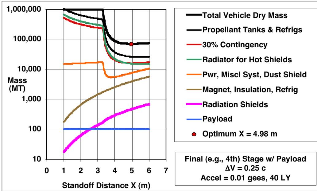
Figure 10. Variation in System Masses with Standoff Distance.
