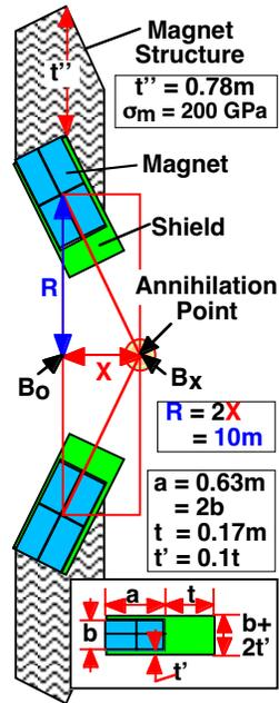
Figure 8. Magnet, Shield, and Magnet Structure Geometry.
