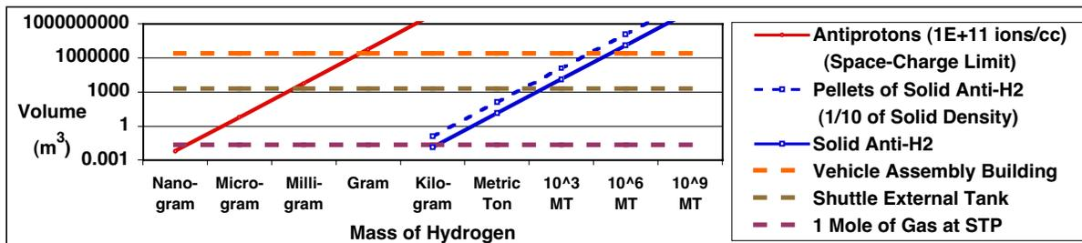
Figure 2. Storage Volume versus Hydrogen Mass for Space-Charge Limited H Ions and Solid H<sub>2</sub> Density.
